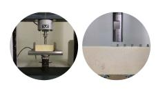
From this experiment, we could developed a special temporary abutment which has lower fracture threshold of less than 200 N (20.4 kgf). It was named as Fuse Abutment. Also it has an anatomic profiles to make temporary prosthetics more esthetic.
