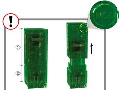
Separate top<sup>1</sup> & bottom<sup>2</sup>, as shown, to reveal inner ampule with fixture
